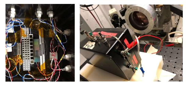
**Figure 4. (left)** Photo of open test box showing the arrangement of the various SiPM arrays. (**right**) Photo experimental testbox showing the test box directly in front of the aperture.
