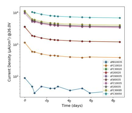
**Figure 8.** Plot of current density as a function of annealing time for all proton irradiated SiPMs. Samples were kept at room temperature between measurements. The one exception to this was during shipping back to NRL.
