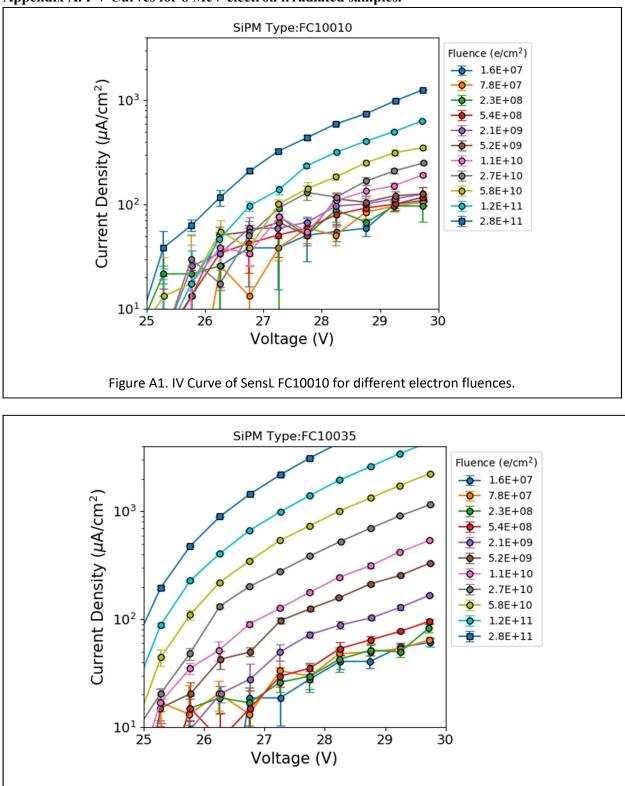
Figure A2. IV Curve of SensL FC10035 for different electron fluences.
