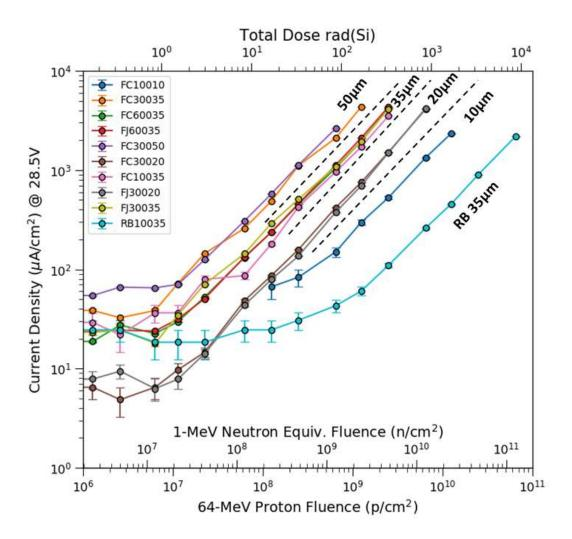
Figure 7. Plot of current density as a function of dose/damage of for all SiPMs biased at 28.5V.
