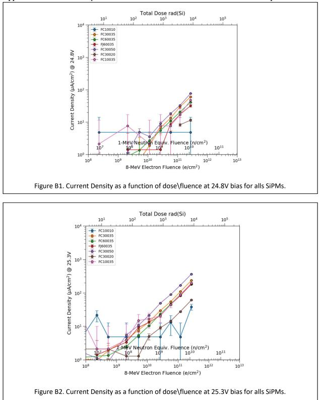
Appendix B. Current density as a function of dose for 8 MeV electron irradiated samples.
