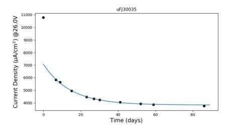
**Figure 9.** Plot shows a fit (blue line) of the annealing data for the SensL FJ30035 where current density is defined by Eq. 3. First point (*t*=0) is excluded from fit.
