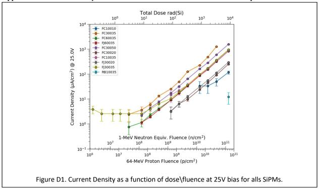
Appendix D. Current Density as a Function of Dose for Proton Irradiated Samples
