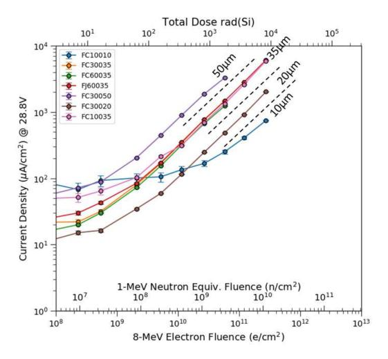
Figure 6. Plot of current density as a function of dose/damage of for all SiPMs biased at 28.8V. SiPMs with the same cell size showed comparable current densities. In general the larger cell size SiPMs showed more susceptibility to radiation damage from a bulk current standpoint. Data collected from 8 MeV electron beam.
