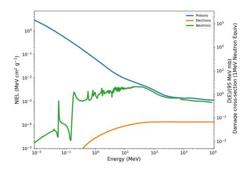
Figure 2. Plot of the NIEL and the displacement damage cross-section for various particles. Note the displacement damage has been normalized by the displacement damage of a 1 MeV neutron. The hardness factor, K, is given by the right axis [16] [17] [18] [19].
