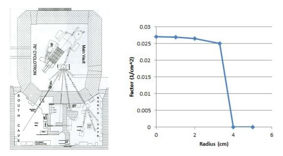
Figure 5. (left) Map of UC Davis Cyclotron Facility. (right) Radial intensity of proton beam at target.
