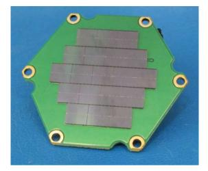
**Figure 1.** Readout board with 19 6 mm SensL SiPMs for a hexagonal SrI<sub>2</sub>:Eu detector used on SIRI-2.
