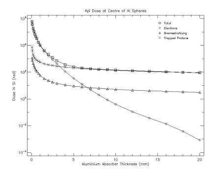
Figure 10. Plot of on-orbit annual dose as a function of Al shielding generated using SPENVIS and SHIELDOSE2 for the SIRI-1 instrument.
