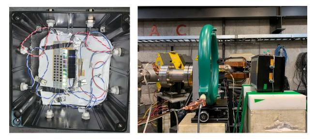
Figure 3. (left) shows the test box used to house the SiPM arrays and the experimental setup in front of the LINAC beam port at the Idaho Accelerator Center.
