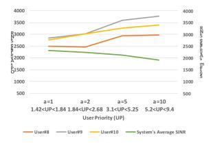
FIGURE 8. The impact of a, both user and average SINR (WSRMax Approach)
