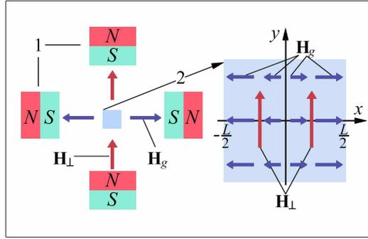
**Figure 5.** Schematic diagram of the system and sources for the uniform and gradient magnetic fields. The electromagnets generating the uniform ( $\mathbf{H}_{\perp}$ ) and gradient ( $\mathbf{H}_g$ ) magnetic fields and the suspension reservoir are marked by 1 and 2, respectively.
