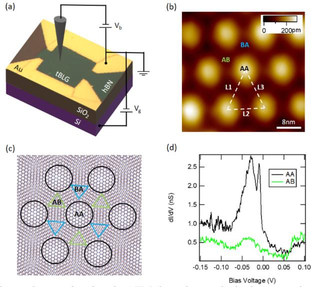
FIG. 1. (a) Schematic of the experimental setup showing the STM tip and an optical microscope image of the measured MATBG sample. (b) Atomic resolution STM topography of the  $1.10^\circ$  moiré superlattice. (c) Schematic of different atomic stacking arrangements arising from the twist of the two layers of graphene. (d)  $dI/dV$  spectroscopy of the MATBG on AA and AB sites of  $1.10^\circ$  moiré when the flat bands are fully filled, where  $V_g = 8$  V.
