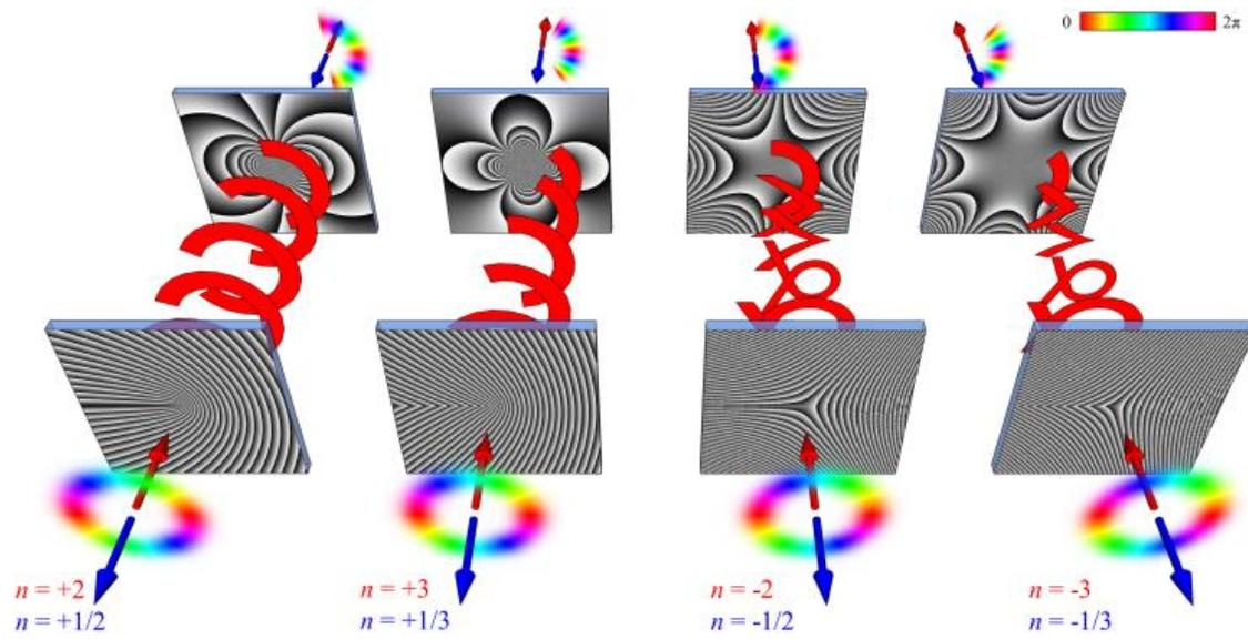
**Figure 1.** Schemes of  $n$ -fold circular-sector transformation of a vortex wavefunction carrying OAM  $\ell=+2$ , for  $n=\{\pm 2, \pm 3\}$  (red arrows direction). The same configurations perform the inverse transformations, i.e.  $n=\{\pm 1/2, \pm 1/3\}$ , when exploited in reverse (blue arrows direction).
