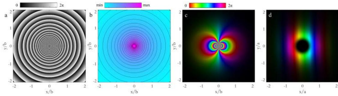
**Figure 4.** Conformal transformation of a dipole field into a linear phase contribution using a circular-sector transformation with factor  $n=+1$ . Comparison between the transformer phase element (a) and the projected potential (b) of a monopole placed at the origin. Input dipole field (c) and output transformed field (d). Brightness and colours refer to intensity and phase, respectively.
