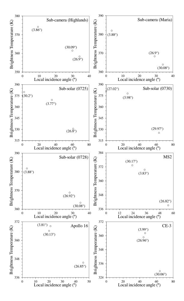
**Figure 6.** Brightness temperature versus local incidence angle for eight typical areas. The two sub-solar points of July 25 and 28 are from nearby homogeneous maria areas to avoid fresh craters which are the exact sub-solar points. Angles in the bracket are phase angles.
