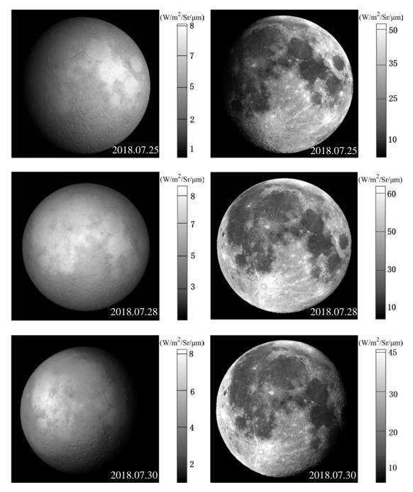
**Figure 1.** The radiance of the Moon imaged by the GF-4 band 6 (left column) and band 5 (right column) for 3 days.
