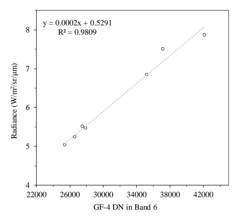
Figure 9. On-board calibration plot of GF-4's band 6.
