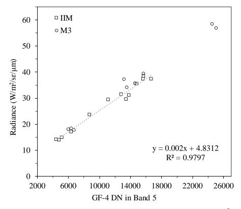
**Figure 7.** On-board calibration plot of GF-4's band 5 using the IIM and  $M^3$  data. The function in the plot was derived from IIM data.
