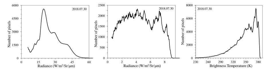
Figure 3. Histograms of VNIR, MIR, and brightness temperature of the lunar disks.
