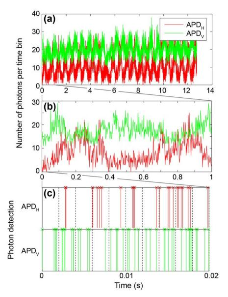
**Fig. 3.** (Color online) (a) Time evolution of single photon detection by  $APD_H$  and  $APD_V$  when the electro-optical phase modulator was driven by a periodic signal (Fig. 1(b,i)). (b) Magnified view of (a). The vertical axis represents the number of photons per time bin (0.002 s). (c) Single-photon detection events in the initial 0.02 s.
