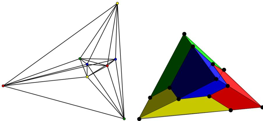
Fig. 1: (Color online) A representation of the smallest tetrahedral color code, in the dual (left) and primal (right) lattice. Colored vertices in the dual correspond to colored cells in the primal, except for the four *quasivertices* furthest from the center
