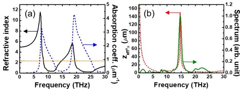
Figure 2: (a) Extraordinary refractive index  $n_{\text{THz}}$  (black line) and absorption coefficient  $\alpha_{\text{THz}}$  (blue dotted line) of cLN, co-plotted with laser group index  $n_g = 2.3$  at 808 nm (orange dotted line). (b) Calculated effective interaction length  $z_{\text{eff,a}}$  (red dotted line) and corresponding radiation spectrum (green solid line) expected from a 35- $\mu\text{m}$ -thick cLN crystal.
