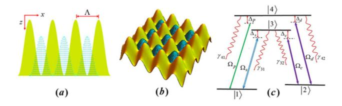
**Fig. 1.** (a) Sketch of 1D optical lattices with the period of  $\Lambda$  along the *x* direction in which the blue area characterizes spatial distribution of the atomic density in dipole traps. (b) Sketch of 2D optical lattices. (c) Schematic diagram of the four-level double-lambda atomic system interacting with four applied fields in a closed-loop transition.
