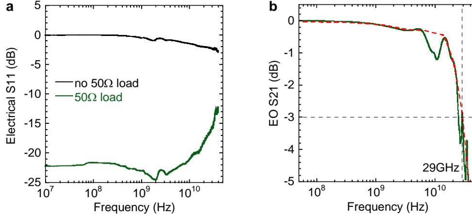
Fig. 5. (a) Electrical S11 parameter as a function of the frequency of the device with (green curve) and without (black curve) 50  $\Omega$  termination. (b) Electro-optical S21 bandwidth of the DLG EAM. The green line is the measured curve, the red dashed line the envelope fit. The measured -3dB bandwidth is  $\sim$ 29GHz mainly limited by the experimental setup loads.
