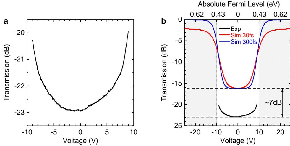
Fig. 4. (a) Optical transmission at 1550nm wavelength as a function of the voltage applied to the DLG capacitor. The transmission is normalized to the fiber to grating insertion loss ( $\sim -11$ dB from the input to the output). (b) Comparison between the measured and simulated transmission as a function of the applied voltage and Fermi level. The dashed areas correspond to the bias regions where the fabricated dielectric suffers breakdown, i.e. above 10V corresponding to 5MV/cm for 20nm SiN.
