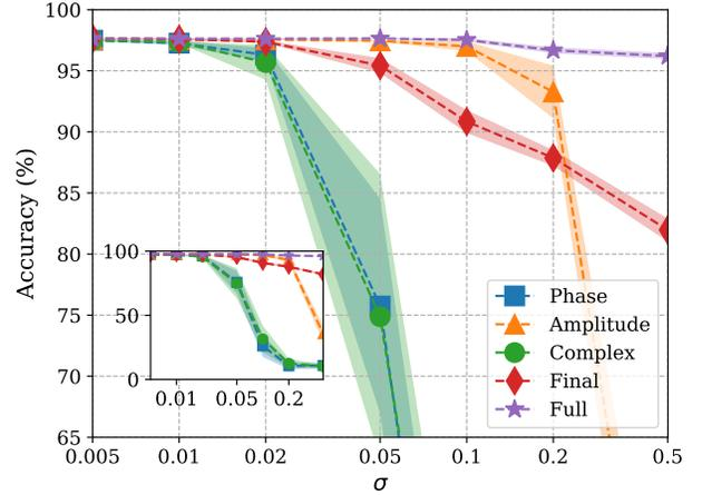
Fig. 5: Degradation in prediction accuracy with increasing noise. Additional phase noise has standard deviation of  $2\pi\sigma$ , while amplitude noise is  $a_\delta = 1 - |\delta|$  with  $\delta$  having standard deviation of  $\sigma$ . “Final” and “Full” indicates restoration of accuracy after re-training the weights of the output layer and the full network when phase noise is added. (Inset) Zoom-out of plot, showing the complete randomization of the network when noise is large.
