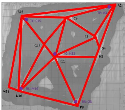
Figure 1: Sketch showing the channel network carved in the PDMS skin, with coordinates of nodes and holes for connecting electrodes. Each letter/number in the coordinate system corresponds to a square with side of 1 cm.
