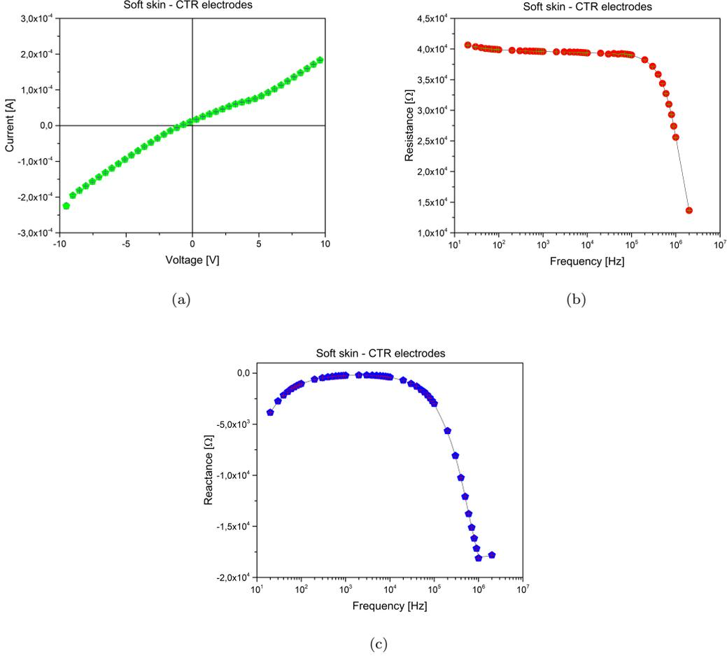
Figure 2: The IV curve (left) and AC impedance measured on conductive liquid at rest, hosted in the random network channel of the soft skin.
