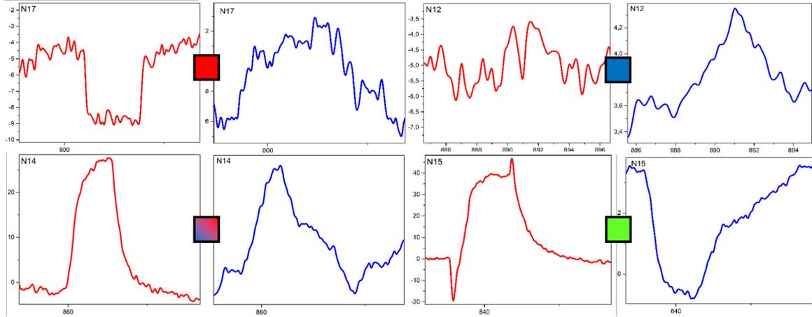
Figure 5: Taxonomy of impedance outputs in response to pressure stimuli, divided into four families. Measurements taken on hard skin with a signal of 100 mV RMS and 1 kHz center frequency.
