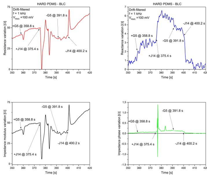
Figure 8: From top left to bottom right: resistance, reactance, impedance modulus and impedance phase output measured from multi-touch experiments performed on the hard skin. Measurements taken at 1 kHz, 100 mV RMS, filtered from drifts by algebraic correction.
