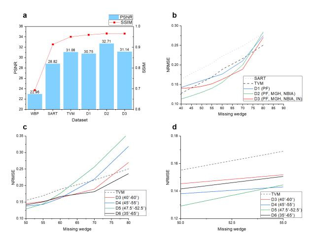
**Fig. 4** | **The performance of IRDM, SART and TVM. a,** Average PSNR and SSIM of SART, TVM, and IRDM trained on datasets D1-D3. **b**, The NRMSE of SART, TVM and IRDM trained on D1-D3. **c,d**, The NRMSE of TVM and IRDM trained on D3-D6.
