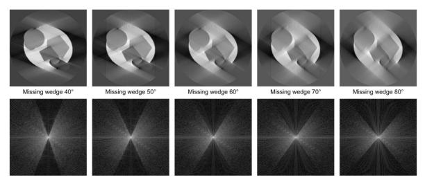
Supplementary Figure 1: WBP reconstruction of 'phantom faces' with different missing wedge angles and their corresponding power spectra.
