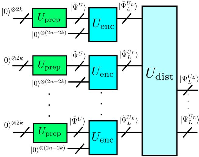
FIG. 4. FT ancilla state distillation circuit for  $|\Psi_L^{UL}\rangle$ . Ancilla states are prepared and encoded via noisy quantum circuits  $U_{\text{prep}}$  and  $U_{\text{enc}}$ . Then they are fed to the distillation circuit and output the qualified ancilla state. The preparation of  $|\Omega_L^{\text{EF}}\rangle$  is similar.
