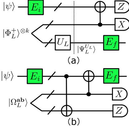
FIG. 3. The effective error model of the Knill (part (a)) and Steane (part(b)) syndrome measurement circuits. While  $E_i$  and  $E_f$  are in general correlated *in time*, they are *spatially* uncorrelated, if the ancilla states are qualified.
