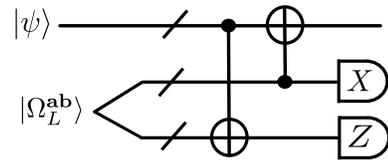
FIG. 2. The quantum circuit for Steane syndrome measurement using an  $[[n, k, d]]$  CSS code. One can simultaneously measure a Hermitian Pauli operator  $i^{\tau_{ab}} X_L^a Z_L^b$ , when the two ancilla blocks are prepared in the state  $|\Omega_L^{ab}\rangle = \frac{1}{\sqrt{2}}(I + i^{\tau_{ab}} X_L^a \otimes Z_L^b) |0_L\rangle^{\otimes k} \otimes |+_L\rangle^{\otimes k}$ .
