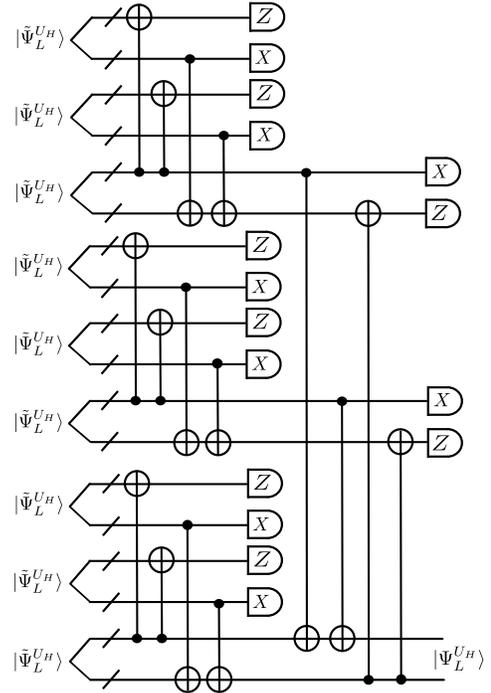
FIG. 6. Two-stage FT ancilla state distillation circuit for  $|\Psi_L^{UH}\rangle$  based on the parity-check matrix of  $[[3, 1, 3]]$  code. This circuit can be used to prepare any logical CSS states up to logical Hadamard gates fault-tolerantly.
