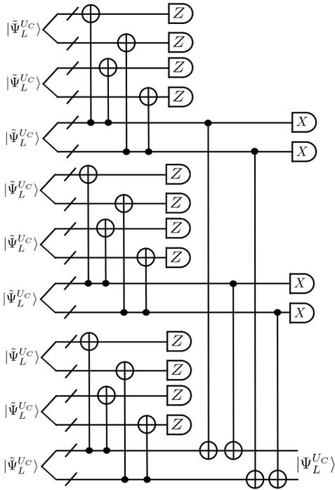
FIG. 5. Two-stage FT ancilla state distillation circuit for  $|\Psi_L^{UC}\rangle$ . The distillation circuit is based on the parity-check matrix of the  $[[3, 1, 3]]$  code for both stages. Actually this circuit can distill any logical CSS states fault-tolerantly.
