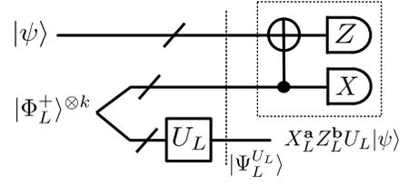
FIG. 1. The quantum circuit for Knill syndrome measurement and gate teleportation for an  $[[n, k, d]]$  stabilizer code. For a logical Clifford circuit  $U_L$ , if  $|\Psi_L^{U_L}\rangle$  is prepared before logical Bell measurement,  $U_L|\psi\rangle$  can be obtained up to some Pauli correction of  $X_L^a Z_L^b$  on the output block, depending on the logical Bell measurement results.
