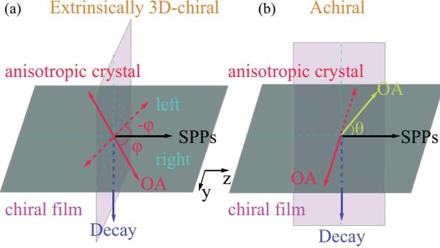
FIG. 4. Origin of chiral sensing: mirror asymmetry of the experimental arrangement. According to the SPP decay direction towards the chiral medium (blue), the SPP momentum (black) and the OA orientation (red), the system is (a) extrinsically 3D-chiral and right-handed when  $0 < \varphi < \pi/2$  and left-handed when  $-\pi/2 < \varphi < 0$  and (b) achiral when  $\varphi = 0$ ,  $\varphi = \pi/2$  and when OA (yellow) lies in the  $xz$  plane.
