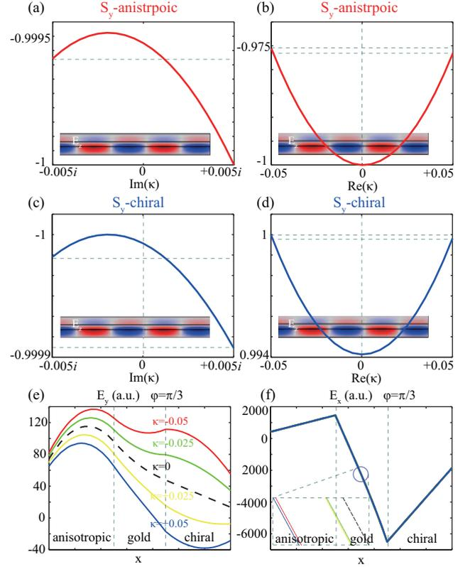
FIG. 5. Transverse SAM ( $S_y$ ) distributions in the system as functions of the real and imaginary part of  $\kappa$ , when  $\varphi = \pi/3$ . (a, c)  $S_y$ - $\text{Im}(\kappa)$  and (b, d)  $S_y$ - $\text{Re}(\kappa)$  in the anisotropic crystal and chiral medium, respectively. (e) Transverse  $E_y$  component distribution and (f) longitudinal  $E_x$  component distribution shows chiral-dependent and -independent behaviors, respectively.
