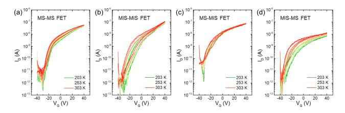
**Fig. S4** *T*-dependent  $I_D$ - $V_G$  characteristics at  $V_D = 0.5$  V for the MS-MS, MIS-MIS, MS-MIS, and MIS-MS FETs. *T* ranges from 203 K (green) to 303 K (red) with a step of 10 K.
