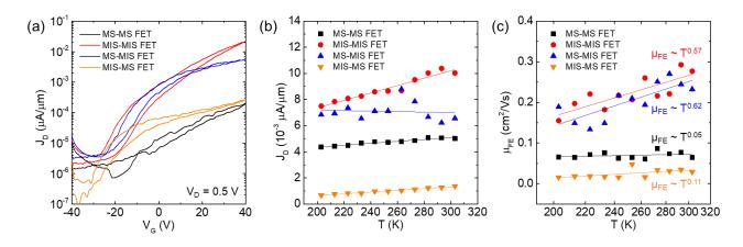
Fig. 5 Comparison of transfer characteristics of MoS<sub>2</sub> FETs with MS and MIS contacts. (a) Room-temperature  $J_D$ - $V_G$  characteristics in logarithmic scale for the MS-MS, MIS-MIS, MS-MIS, and MIS-MS MoS<sub>2</sub> FETs at  $V_D = 0.5$  V. (b) The maximum  $J_D$  obtained at  $V_G = 40$  V as a function of T for all the types of the FETs. (c) The maximum  $\mu_{FE}$  as a function of T in logarithmic scale for all the types of the FETs.
