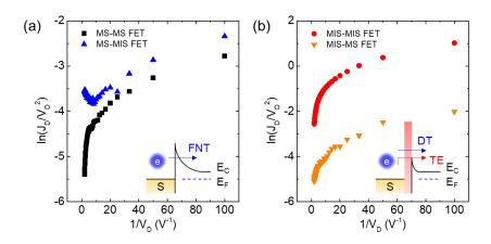
Fig. 4 Impact of MS and MIS drain contacts on the carrier injection at the source. (a, b) Comparison of  $\ln(J_D/V_D^2)$  versus  $1/V_D$  curves at  $V_G = 40$  V for the MS-source FETs (including the MS-MS and MS-MIS FETs) and the MIS-source FETs (including the MIS-MIS and MIS-MS FETs), respectively. Inset: Energy band diagram illustrates the FNT dominating in the MS-MIS FET, in a comparison with the DT and TE dominating in the MS-MS, MIS-MIS, and MIS-MS FETs.
