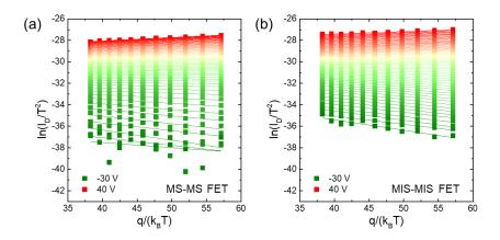
**Fig. S5**  $\ln(I_D/T^2)$  versus  $q/(k_BT)$  plots for (a) the MS-MS FET and (b) the MIS-MIS FET with the T ranging from 203 to 303 K. The value of the SBH is extracted from the linear fit as a function of  $V_G$  ranging from -30 V (green) to 40 V (red).
