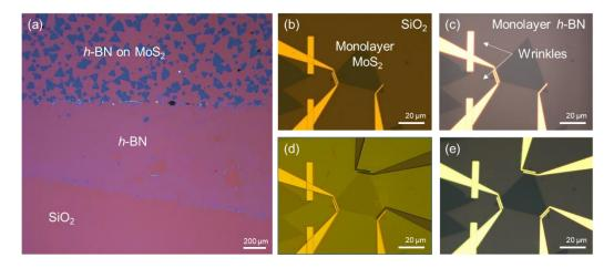
**Fig. S1** (a) Optical microscope image of an h-BN/MoS<sub>2</sub> heterostructure on SiO<sub>2</sub>/Si substrate. The monolayer MoS<sub>2</sub> and monolayer h-BN are wet-transferred on the substrate sequentially. (b-e) Optical microscope images show the process to fabricate the MS-MS, MS-MIS (MIS-MS), and MIS-MIS FETs on a single monolayer MoS<sub>2</sub> triangular domain.
