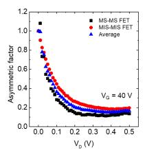
**Fig. S2** Asymmetric factor versus  $V_D$  for the MS-MS and MIS-MIS FETs at  $V_G = 40$  V and the average value. The asymmetric factor is defined as the ratio of the magnitude of the current density at the positive  $V_D$  to that at the negative  $V_D$ .
