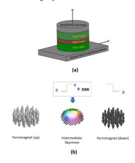
Fig. 1: (a) Schematic presentation of a Magnetic Tunnel Junction and (b) Skyrmion mediated switching scheme
