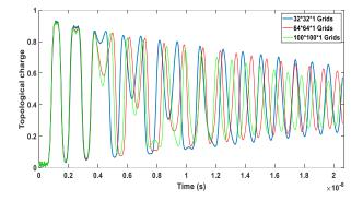
Fig. 5: Evolution of topological charge of 100nm MTJ for  $32\times32\times1$ ,  $64\times64\times1$  and  $100\times100\times1$  Grids
