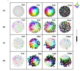
Fig. 4: Magnetization states visited at different time of 20 nm nanomagnets for (a) non-thermal switching (b) thermal switching, (c) and (d) error cases.
