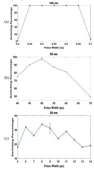
Fig. 3: Switching probability vs pulse width of (a) 100nm (b) 50nm and (c) 20 nm nanomagnets.
