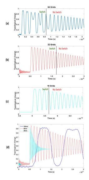
Fig. 2: "Switch" and "no switch" region without thermal perturbation for (a) 100nm (b) 50 nm (c) 20 nm and (d) Comparison of topological evolution of three nanomagnets using same time scale for the nanomagnets of three different sizes.
