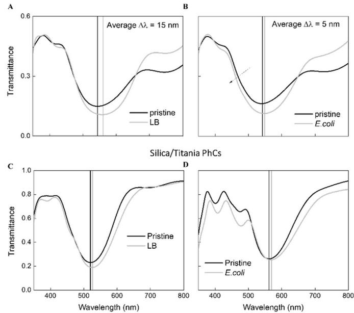
Figure 4. (A) Average transmittance spectrum of Ag/1D photonic crystals upon exposure to the LB medium and (B) to *E. coli*. (C) Average transmittance spectrum of 1D photonic crystals (without silver layer) upon exposure to the LB medium and (D) to *E. coli*. Data were averaged over two sets of measurements (six samples per measurement).
