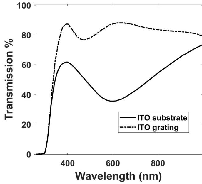
Figure 1. Transmission (%) spectra of the ITO substrate (dash-dotted curve) and of the ITO grating (solid curve).
