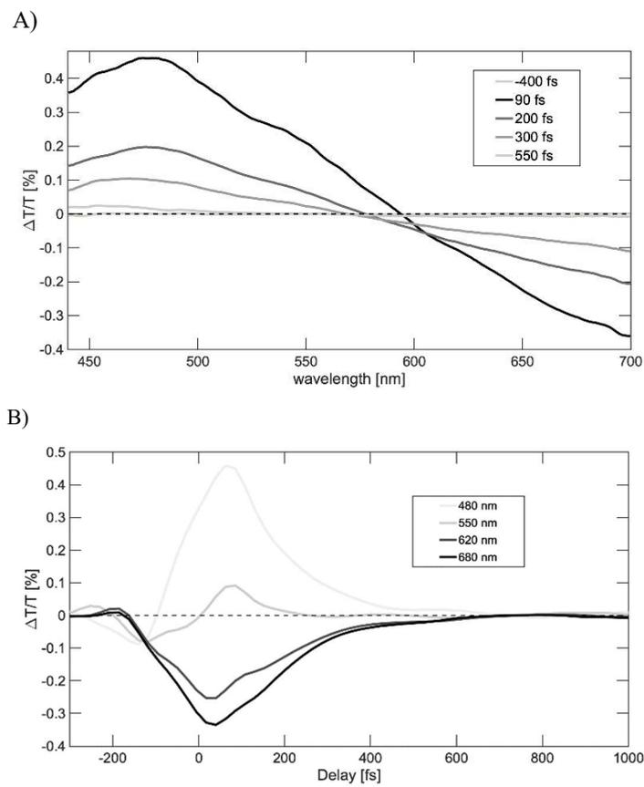
Figure 2. (A) Differential transmission spectra at different time delays of the ITO grating; (B) Differential transmission dynamics at different wavelengths of the ITO grating.
