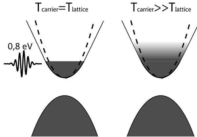
Figure 3. Sketch of the carrier distribution in the conduction band of ITO upon excitation in the near-infrared.
