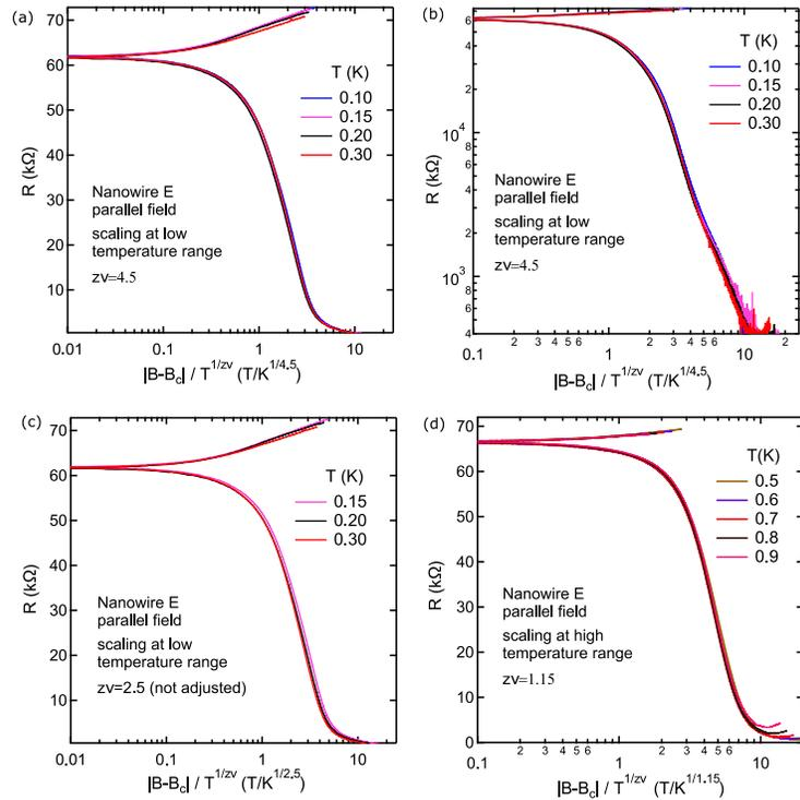
**Fig. 3.** The scaling plot of the resistance of nanowire E in parallel magnetic fields. (a) The scaling at low temperatures near the crossing field  $B_{cL} = 11.7$  T. The exponent has been adjusted to give the best data collapse. (b) The same scaling on log-log scale. (c) The same scaling at with fixed exponent  $z\nu = 2.5$  and  $R(B)$  curve at  $T = 100$  mK not included. (d) The scaling at higher temperatures near the second crossing field  $B_{cH} = 12.5$  T.
