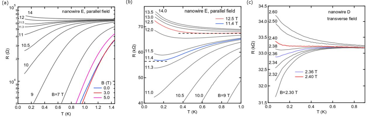
**Fig. 1.** (a) Resistance versus temperature dependence for nanowire E in parallel magnetic field. (b) Same data in the transition range at high fields. The dashed lines indicate resistance at which  $R(T)$  changes from superconductor-like to insulator-like behavior at low ( $T < 0.25\ \text{K}$ ) and higher ( $0.4 < T < 1\ \text{K}$ ) temperatures. (c) Resistance versus temperature in the transition range for nanowire D in transverse magnetic field.
