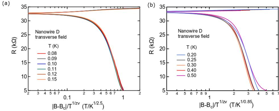
**Fig. 4.** The scaling plot of the resistance of nanowire D in transversel magntic fields. (a) The scaling at low temperatures near the crossing field  $B_{cL} = 2.37$  T. (b) The scaling at higher temperatures near the second crossing field  $B_{cH} = 2.45$  T.
