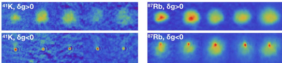
FIG. 6. (a) Absorption images (frame size:  $190 \times 190 \mu\text{m}$ ) of  $^{41}\text{K}$  and  $^{87}\text{Rb}$  for different values of TOF. For  $^{41}\text{K}$  from left to right: TOF=17.5, 19.5, 21.5, 23.5, 25.5 ms. For  $^{87}\text{Rb}$  from left to right: TOF=20, 22, 24, 26, 28 ms. Top panels correspond to  $a_{12} \simeq -18a_0$  ( $\delta g > 0$ ), and bottom panels to  $a_{12} \simeq -85a_0$  ( $\delta g < 0$ ).
