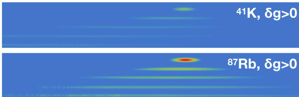
FIG. 8. Simulated density distributions (frame size:  $6 \times 155 \mu\text{m}$ ) of  $^{41}\text{K}$  and  $^{87}\text{Rb}$  for  $a_{12} = -12a_0$  ( $\delta g > 0$ ), at different evolution times  $t$  in the waveguide. For both species, from top to bottom  $t = 0, 10, 20, 30, 40$  ms;  $N_1 = 1.5 \times 10^3$  and  $N_2 = 4 \times N_1$ .
