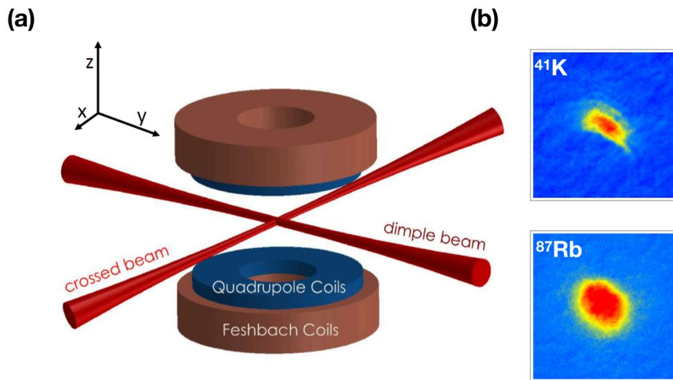
FIG. 1. (a) Schematics of the experiment, showing the optical dipole trap (ODT) beams, quadrupole and Feshbach coils. (b) Absorption images of the dual-species Bose–Einstein condensate (BEC). Images are taken after 18 ms of TOF for  $^{41}\text{K}$  and 20.5 ms for  $^{87}\text{Rb}$ .  $N_{\text{K}} \sim 2 \times 10^4$  and  $N_{\text{Rb}} \sim 6 \times 10^4$ . During TOF expansion, the Feshbach field is set at 77.5 G, corresponding to  $a_{12} \simeq 255a_0$ .
