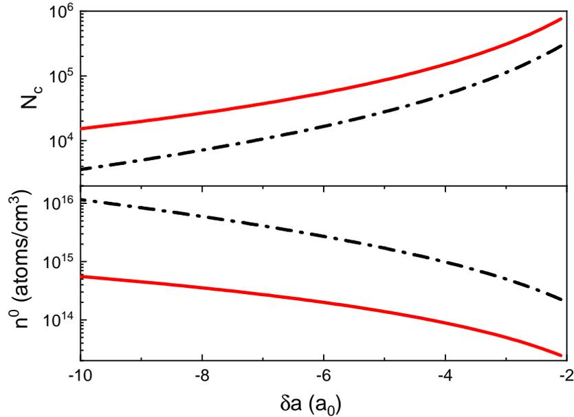
FIG. 5. Calculated critical atom number  $N_c$  (top panel) and droplet density (bottom panel) in logarithmic scale as a function of  $\delta a$  for the  $^{41}\text{K}$ - $^{87}\text{Rb}$  mixture (solid red lines) and the  $^{39}\text{K}$  spin mixture (dash-dotted black lines).
