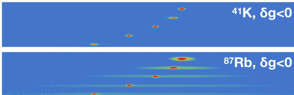
FIG. 9. Simulated density distributions (frame size:  $6 \times 155 \mu\text{m}$ ) of  $^{41}\text{K}$  and  $^{87}\text{Rb}$  for  $a_{12} = -83a_0$  ( $\delta g < 0$ ), at different evolution times  $t$  in the waveguide. For both species, from top to bottom  $t = 0, 10, 20, 30, 40$  ms;  $N_1 = 1.5 \times 10^3$  and  $N_2 = 4 \times N_1$ .
