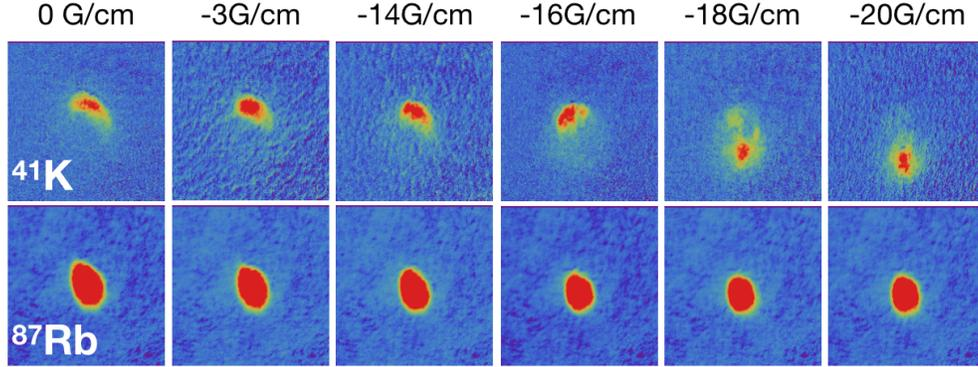
FIG. 3. Absorption images of the dual-species BEC for different values of  $b_z$ . During TOF expansion, the Feshbach field is set at 77.5 G corresponding to  $a_{12} \simeq 255a_0$ .
