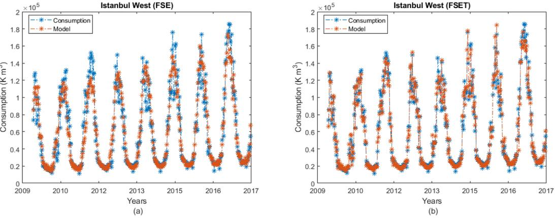
**Figure 5:** Weekly forecasting for Istanbul West using (a) FSE and (b) FSET
