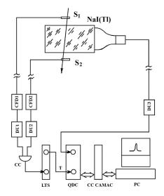
**Fig. 2.** The block diagram of calibration of the extended quadrahedral NaI(Tl) spectrometer:  $S_1$  and  $S_2$  – trigger scintillation counters; NaI(Tl) – extended quadrahedral spectrometer; CFD1 and CFD2 – constant-fraction discriminator; DU1 – DU3 – delay unit; CC – coincidence circuit; LTS – long time signal shaper; T – trigger (T =  $S_1$ · $S_2$ ); QDC – charge-to-digital converter; CC CAMAC – crate-controller CAMAC; PC - personal computer.
