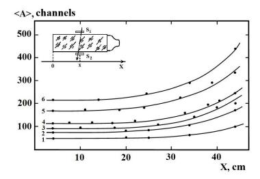
**Fig. 3.** Dependence of average amplitude of the signal of the extended quadrahedral NaI(Tl) spectrometer from the voltage on the voltage divider PMT-52: 1-U = 1100 V; 2-U = 1180 V; 3-U = 1217 V; 4-U = 1260 V; 5-U = 1305 V; 6-U = 1355 V.
