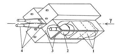
**Fig. 1.** The diagram of the set-up for studying the total photoproduction cross-section of neutral pions near the threshold on neutrons: 1-blocks of extended quadrahedral NaI(Tl) spectrometers; 2 – PMT-52; 3 – frame; 4 – scintillation counters of anticoincidence.
