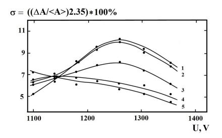
**Fig. 4.** Dependence of the energy resolution of the extended quadrahedral NaI(Tl) spectrometer's from the voltage on the PMT-52 voltage divider and the entry point of the cosmic muon into the spectrometer (insert Fig. 3): x = 4 cm; x = 22 cm; x = 38 cm; x = 40 cm; x = 44 cm.
