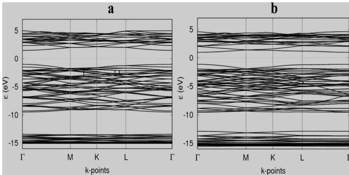
**Figure 11.** The calculated band structures at high symmetry k-points for complex system of B doped mg decorated graphene sheet. Gr-B-Mg configuration 1 (a) , Gr-B-Mg configuration 1 (b) .
