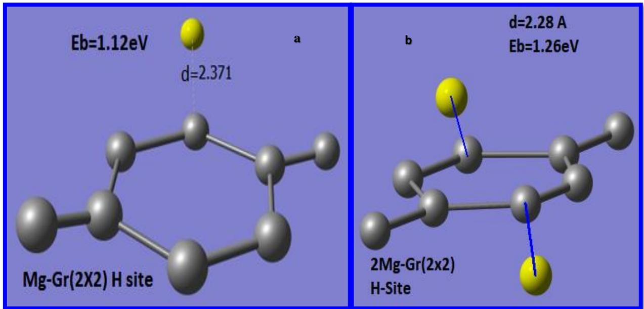
Fig.8. The optimized structure of single Mg atom (a) and double Mg atom (b) adsorbed on the H site of the (2X2) cell of graphene Mg -Gr(2X2)
