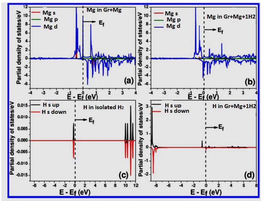
**Figure 6.** Partial density of states (PDOS)  $1\text{H}_2/\text{Mg}/\text{B}/\text{Gr}$  complex system.
