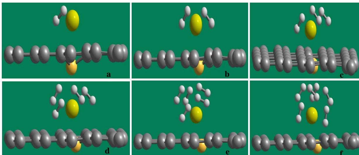
Fig.4 a-f. The optimized structures of H<sub>2</sub> molecules adsorbed on Mg/B/Graphene side view-II
