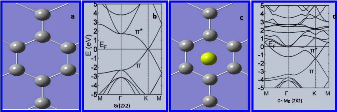
Figure 7. Gr (2X2) and Mg decorated Gr (2X2) with periodic boundary condition.
