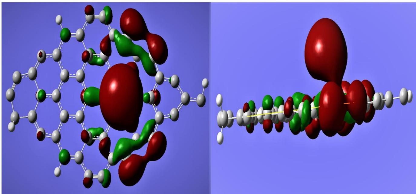
Figure 9 :Gr (4X4) B doped Mg coated complex system (a)HOMO Front view & (b)HOMO side view at MO=155;ISOVALU=0.02
