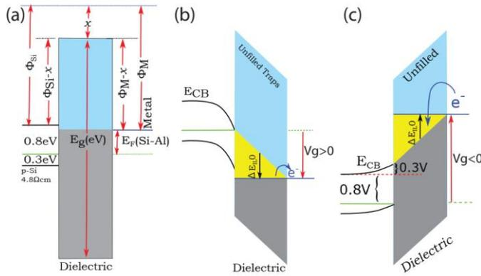
Fig. 2. Energy band diagram of the MIS devices at different biasing condition. (a) Illustration of flatband condition before applying any potential. (b) During discharge of electronic traps a positive gate voltage ( $V_g > 0$ ) is applied, where, the yellow shaded region indicating the accessible traps in the dielectric. (c) The band bending during injection of electron to trap states due to negative gate bias ( $V_g < 0$ ) for a longer time.
