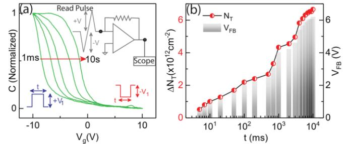
Fig. 3. (a) The CV curve is measured on  $\text{HfO}_2$  based MIS devices after application of every injection voltage pulse ( $-V_1 = -10$  V) till 10 s. Inset: The CV curve was measured by applying the triangular voltage pulses. (b) Change in  $V_{FB}$  and  $\Delta N_T$  due to application of  $-V_1$  at different time ( $t = 1-10^4$  ms).
