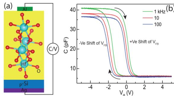
Fig 1: (a) Schematic structure of MIS device with  $\text{HfO}_2$  film on silicon substrate (p-Si). The molecular structure is created by using the VESTA (<https://jp-minerals.org/>). (b) The CV curve was measured at different frequency domain by sweeping the gate potential from  $-5 \text{ V}$  to  $+5 \text{ V}$  and back.
