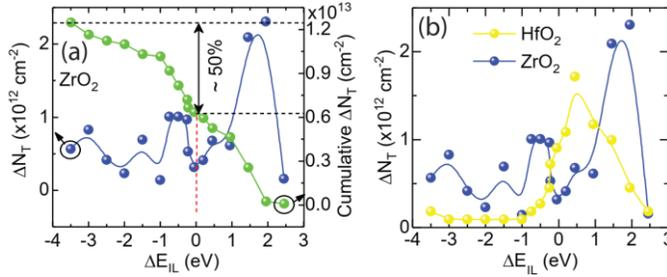
Fig. 6. (a) Distribution of traps energy and cumulative trap density at different energy levels for ZrO<sub>2</sub> dielectric. 50 % of traps are located above the Si-E<sub>CB</sub>. (b) Comparison of trap energy spectrum for HfO<sub>2</sub> and ZrO<sub>2</sub> dielectric.
