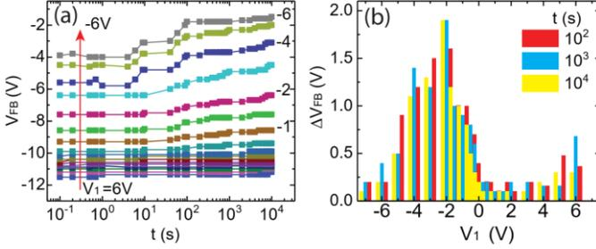
Fig. 4. (a) Different flatband position due to injection of charge to HfO<sub>2</sub> dielectric by applying the injection voltage ( $V_1$ ) from 6 V to -6 V for  $10^4$  s. (b) Shift  $\Delta V_{FB}$  with respect to  $V_1$  measured for different injection time.
