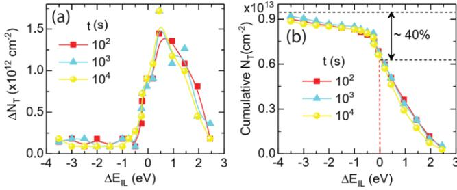
Fig. 5. (a) Spectral energy distribution of electronic trap state compared for different injection time for HfO<sub>2</sub> dielectric. (b) A cumulative trap density is extracted with respect to energy level of traps for the different injection time.
