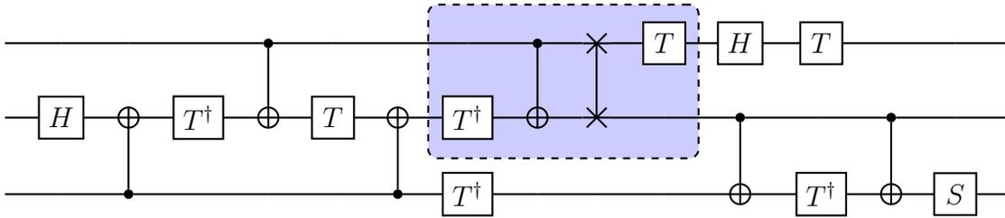
Figure 8: CCNOT with nearest-neighbor connectivity, placing a SWAP on the top two qubit lines. The entire highlighted subcircuit may be translated to at most 3 CNOT gates.
