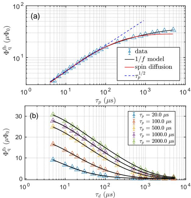
FIG. 3: Measurements of  $\Phi_q^{\text{fb}}$  versus time for (a) polarization and (b) depolarization experiments at  $T = 12.5$  mK. In panel (a)  $\tau_d$  is fixed at  $1 \mu\text{s}$ . In both panels, the solid black curves show best fits to Eq. (7) assuming dynamics governed by the empirical model given by Eq. (5). The dashed line in (a) represents  $\sqrt{\tau_p}$ -dependence and the solid red curve is obtained from spin diffusion model (Eq. (D12)) as described in the text.
