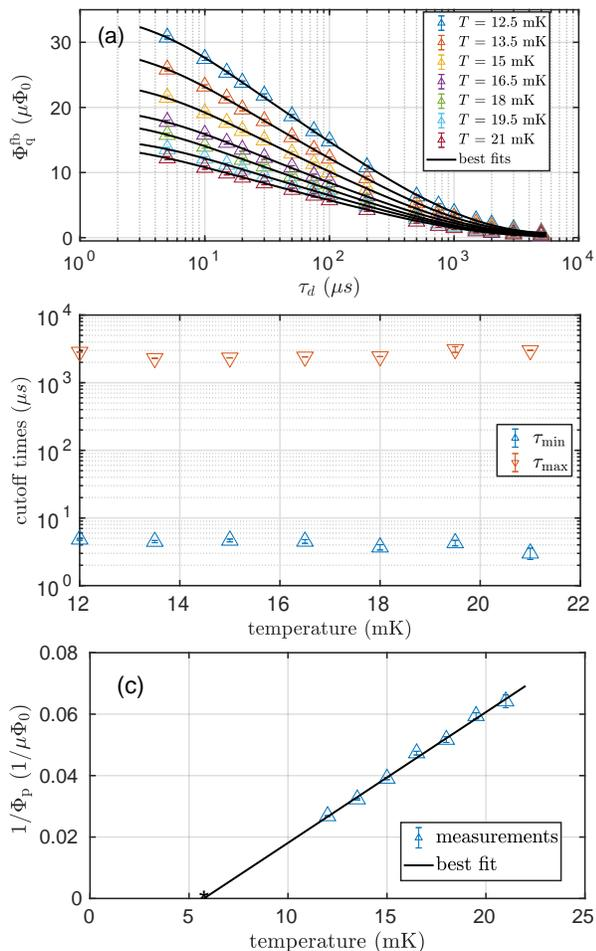
FIG. 4: (a) Measurements of  $\Phi_q^{\text{fb}}$  for a range of temperatures. The data shown are from a protocol that varied  $\tau_d$  and fixed  $\tau_p = 2$  ms. The solid lines show best fits to Eq. (7) using  $1/f$  model with parameters  $\tau_{\text{min}}(T)$  and  $\tau_{\text{max}}(T)$  shown in (b) and  $\Phi_p(T)$  shown in (c). From the fit to the Curie-Weiss model, we estimate a critical temperature  $T_c = 5.7 \pm 0.3$  mK.
