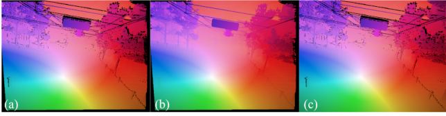
Fig. 7: Optical flow with masks. (a) Both masks. (b) Out-of-FOV mask only. (c) Occlusion mask only.
