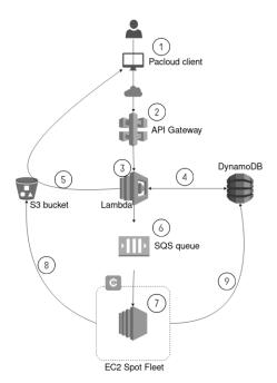
Figure 1. Server-Side Architecture Design
