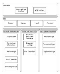
Figure 7. Client-Side Architecture
