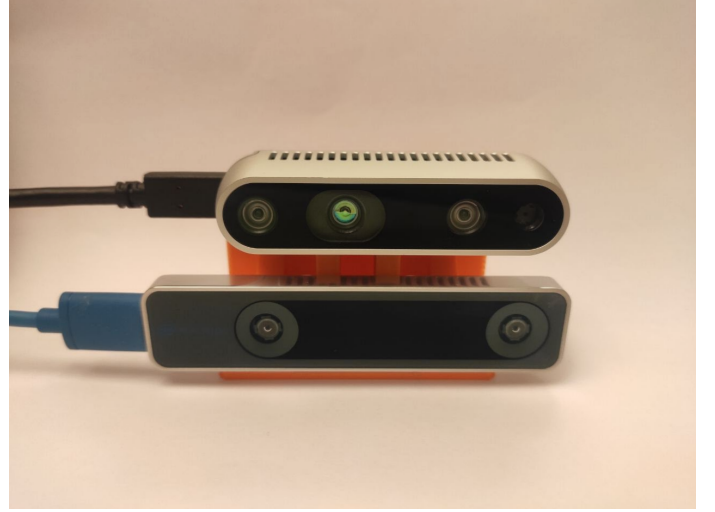
Fig. 1: Sensor suite. Intel RealSense D435i RGBD (top). Intel Realsense T265 tracking camera (bottom) Designed mount provides known and constant transformation between cameras.
