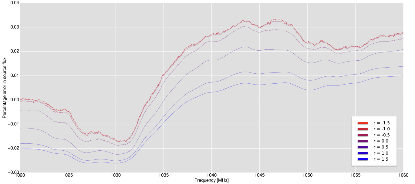
Figure 9. A subset of the MeerKAT L-band simulation showing the percentage error in the spectrum of a target source as a function of frequency, for seven different values of the robust parameter. The robust parameters are colour coded as per the legend.
