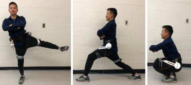
Fig. 4. Demonstration of the range of motion of the robot. The hip exoskeleton is designed with large ranges of motion to support the wearer to perform various activities.
