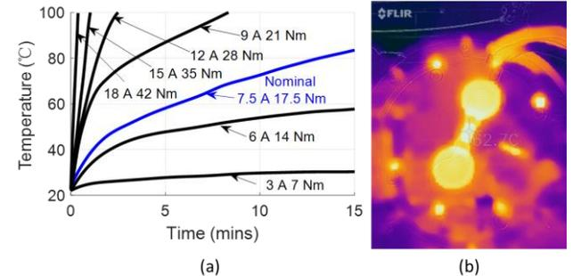
Fig. 10. (a) Stator temperature over time for different current conditions; (b) Thermal image after 15 min of continuous 7.5 A current operation. The actuator surface reached the maximum temperature of 62.7 °C.
