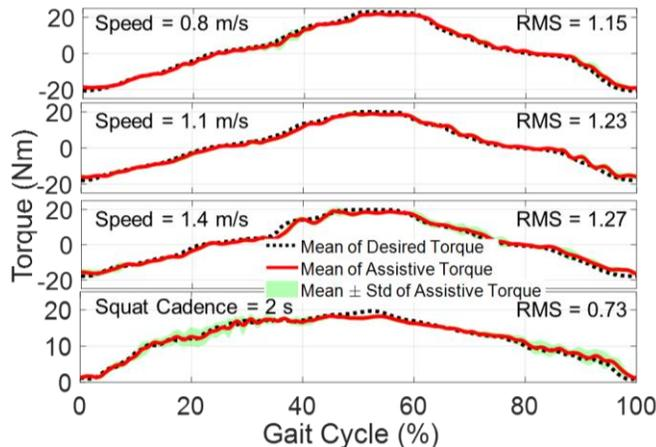
Fig. 13. Torque tracking performance of  $\pm 20$  Nm assistance during walking and squatting tests. The mean of actual assistive torque (red) tracked the desired torque (black dash) well. The RMS errors of torque tracking (0.8 m/s, 1.1 m/s and 1.4 m/s walking, 2 s cadence squatting) were 1.15 Nm, 1.23 Nm, 1.27 Nm and 0.73 Nm respectively (5.75%, 6.15%, 6.35% and 3.65% of the peak torque). The tracking accuracy is superior to the SEA based exoskeleton ( $\pm 10$  Nm and 21.5 % error) [16].
