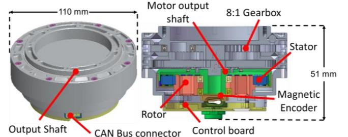
Fig. 3. The fully-integrated quasi-direct drive actuator consists of a high torque density motor, an 8:1 gearbox, a magnetic encoder, and control electronics. The motor is designed to be compact ( $\Phi 110 \text{ mm} \times 52 \text{ mm}$  height), lightweight (777 g), and able to generate high torque ( $17.5 \text{ Nm}$  nominal torque and  $42 \text{ Nm}$  peak torque).
