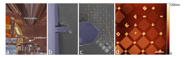
**Figure 2:** Correlative imaging in process on silicon micro-pillars. a) Optical image showing how the AFM cantilever is positioned at the end of a low-profile, overhanging structure that fits between the pole piece and the sample. b) & c) The cantilever (colourized in purple on the HIM images) can be navigated by making use of the large FOV image provided by the HIM. d) AFM height image of Si nano-pillars taken in off-resonance tapping mode. Scale bar 5 µm.
