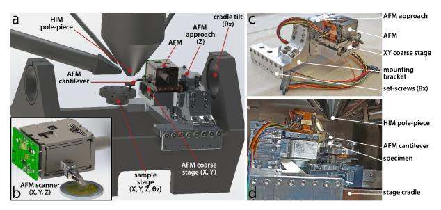
**Figure 1**: AFM assembly and integration inside a Zeiss ORION NanoFab Helium Ion Microscope. a) Simplified CAD rendering of the AFM assembly mounted onto the HIM cradle and b) detailed view of the AFM scan head and a 2€ coin for scale. c) Annotated photograph of the AFM assembly and d) after being mounted inside the chamber of the HIM.
