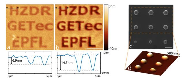
**Figure 3:** AFM height images of Poly(methyl methacrylate) after exposure to a)  $1 \times 10^{13}$  and b)  $3 \times 10^{13}$  He ion cm<sup>-2</sup>. Image is taken in off-resonance tapping mode, scale bar 4 µm. c) Silicon bubbles imaged with HIM and d) AFM (off-resonance tapping mode, scale bar 1 µm.)
