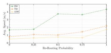
Figure 7. Average speed as a function of the re-routing probabilities for Berlin and different maximum number of vehicles.
