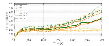
Figure 2. Number of vehicles for the uncapped scenario for London, as a function of time and different insertion rates.
