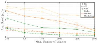
Figure 5. Capped scenario for Manhattan, London and Berlin. Average speed as a function of the number of vehicles.
