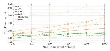
Figure 6. Capped scenario for Manhattan, Rome and Berlin. Average trip time as a function of the number of vehicles.
