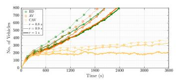
Figure 1. Number of vehicles for the uncapped scenario for Paris, as a function of time and different insertion rates.
