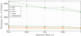
Figure 4. Number of vehicles for the uncapped scenario for Paris and Manhattan, as a function of the different insertion rates.
