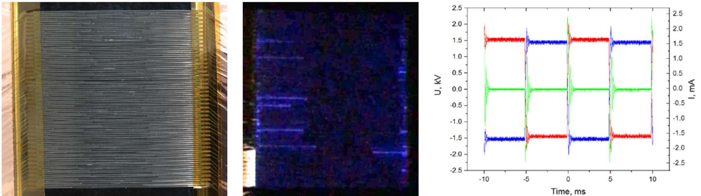
Figure 3. The design of the electrodes of the barrier discharge layer (left); plasma emission at maximum test voltage of 4 kV (center); voltage and current through the discharge device in the design regime (right). Red and blue lines represent voltage on the adjacent electrodes, green line - total current.
