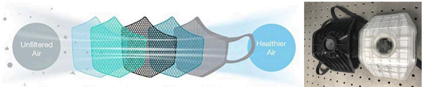
Figure 1. The standard sequence of layers in N-95/N-99 masks (left); N-99 half-face respirator (right).
