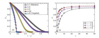
FIG. 3. Results for SF networks. Comparison of theory (lines) and simulation (symbols) for limited knowledge immunization or attack, n, for SF networks. (a) The size of the giant component versus n for SF network with  $\gamma = 2.5$ . (b) Critical threshold  $p_c$  versus n on SF networks. Simulations are obtained for a system with  $10^6$  nodes and averaged over 100 independent realizations. The minimum and maximum degree of network are m = 2 and K = 1000 respectively.
