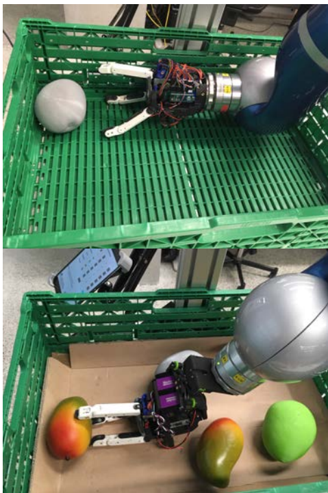
Fig. 1: Without Wrist Wallgrasp works only for quite empty IFCO on one wall - with wrist on all walls and in crowded scenarios
