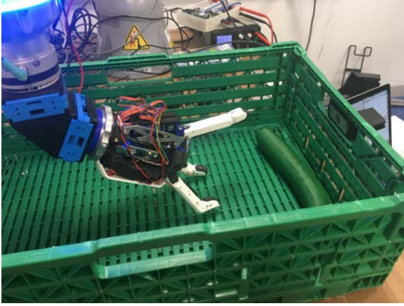
Fig. 2: CLASH mounted with 60 degree rotation adapter on KUKA IIWA
