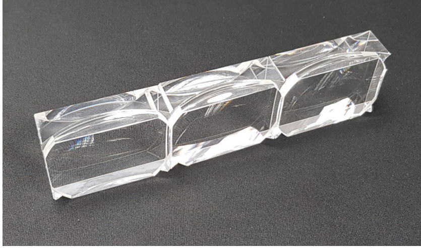
Figure 2: Three focusing lens triplets, each a lanthanum crown glass lens between two fused silica pieces with flat outer surfaces, focus the light from the radiator bar on the back side of the prism.
