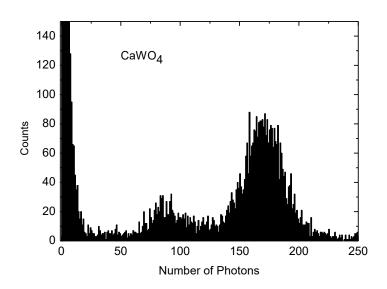
Fig. 8. Histogram of number of photons recorded by the light channel of the CPSD with a CaWO<sub>4</sub> scintillator irradiated by a <sup>57</sup>Co  $\gamma$ -source. The contributions to the histogram are the same as for the energy spectrum of the phonon channel.
