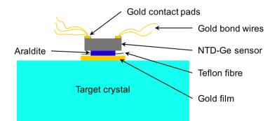
Fig. 2. Schematic of the phonon detector layout.
