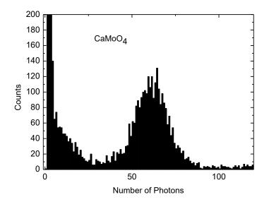
Fig. 9. Histogram of number of photons recorded by the light channel of the CPSD with a CaMoO<sub>4</sub> scintillator irradiated by a  ${}^{57}$ Co  $\gamma$ -source.
