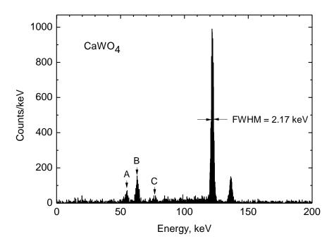
Fig. 6: Energy spectrum recorded by the phonon channel of the CPSD with a CaWO<sub>4</sub> absorber irradiated by a <sup>57</sup>Co  $\gamma$ -source. The escape peaks A (122.1 keV – W-K<sub> $\beta$ </sub>), B (122.1 keV – W-K<sub> $\alpha$ </sub>), and C (136.5 keV – W-K<sub> $\alpha$ </sub>) are due to tungsten K<sub> $\alpha$ </sub> and K<sub> $\beta$ </sub> gamma having a significant probability of leaving the absorber crystal.
