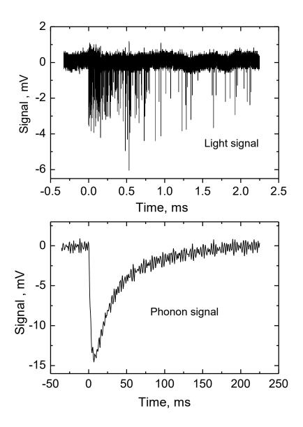
Fig. 14. Typical waveforms of the signals recorded by light (top) and phonon (bottom) channels of the CPSD following deposition of 122.1 keV  $\gamma$ -quanta in CaWO<sub>4</sub>. Note a two order of magnitude difference of the time scale for the two plots.
