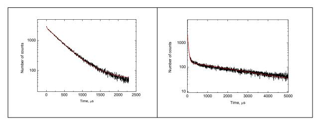
Fig. 10 Scintillation decay curves of CaWO<sub>4</sub> (left) and CaMoO<sub>4</sub> (right) measured at a temperature of 18 mK. The red lines show the best fit to the experimental data using the sum of two exponential functions:  $y = A_f \exp(-\tau_f^{-1}t) + A_s \exp(-\tau_s^{-1}t) + y_0$ .
