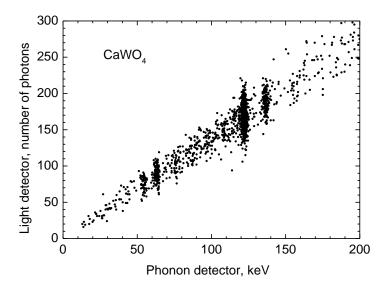
Fig. 11. Scatter plot of the energy in the light channel versus the energy in the phonon channel measured with a CPSD with CaWO<sub>4</sub> scintillator irradiated by a  ${}^{57}$ Co  $\gamma$ -source.
