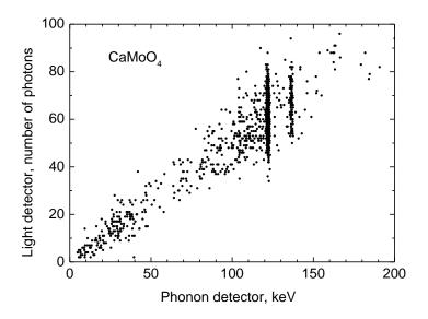
Fig. 12. Scatter plot of the energy in the light channel versus the energy in the phonon channel measured with a CPSD with CaMoO<sub>4</sub> scintillator irradiated by a  ${}^{57}$ Co  $\gamma$ -source.
