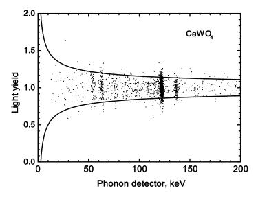
Fig. 13. Light yield versus energy of events. The solid lines indicate the 90% significance band of the electron recoil band at yield = 1.
