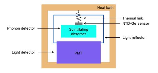
Fig. 1. Schematic view of the detector module.
