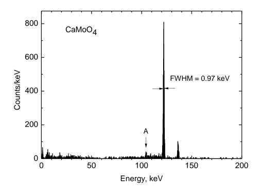
Fig. 7: Energy spectrum recorded by the phonon channel of the CPSD with a CaMoO<sub>4</sub> absorber irradiated by a <sup>57</sup>Co  $\gamma$ -source. The escape peak A (122.1 keV – Mo-K<sub> $\alpha$ </sub>) is visible but less prominent than in tungsten due to molybdenum K-energies significantly lower and thus gamma less likely to leave the absorber crystal. Other escape peaks are too weak to be visible.
