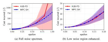
Fig. 1: Performance comparison of HJB-FD and MPC-SH on the 1-D nonlinear system for different noise levels.
