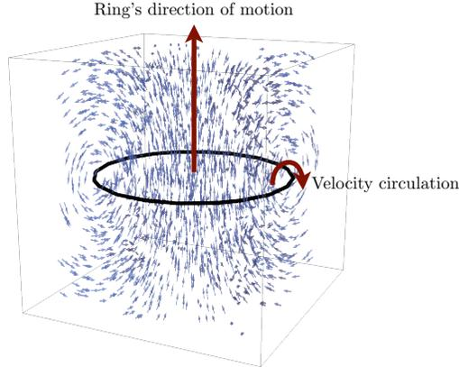
Figure 4: Cartoon of the velocity flow around a vortex ring moving in the  $z$  direction. Note that the fluid velocity is such that it flows through the ring in the same direction that the ring is moving. The flow then circulates around the ring as shown.
