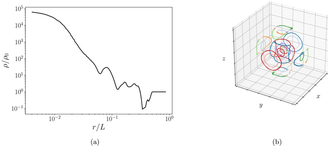
Figure 7: Numerical simulation of a halo formed from the collapse and merger of a symmetric configuration of four Gaussian peaks (see text for details). **a.** Spherically averaged density profile (as a function of radius) of the virialized halo that forms from the coalescence of the peaks. **b.** Vortex rings formed in the same halo.
