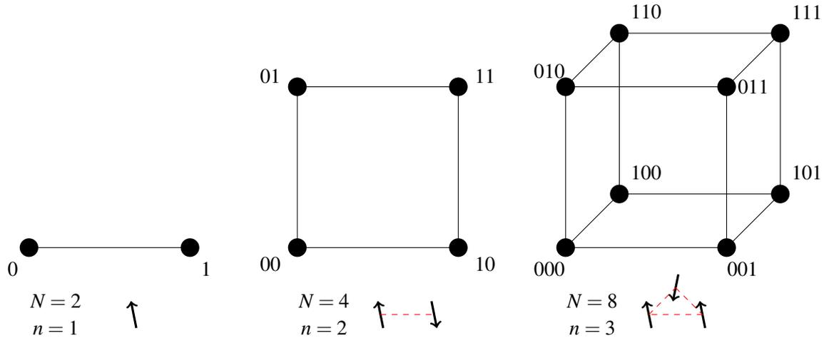
Figure 7: Hypercubes and qubits for  $n = 1, 2, 3$ , showing the encoding from quantum walk graph (upper) of size  $N = 2^n$  to qubit graph (lower) of size  $n$ . The red dotted lines indicate possible interaction terms between qubits, that can be used to encode problems into Hamiltonians.
