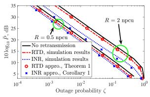
Fig. 4. Minimum required power without optimized power allocation (23) under various outage probabilities,  $\sigma = 0.8$ , R = 0.5, 2 npcu.
