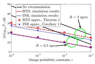
Fig. 3. Minimum required power under various outage constraints for the RTD and the INR,  $\sigma=0.8,\,R=0.5,2$  npcu.
