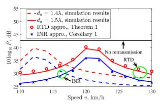
Fig. 5. Minimum required power for the RTD and the INR with given outage constraint, for different speed v. R=3 npcu,  $\epsilon=10^{-3}$ .
