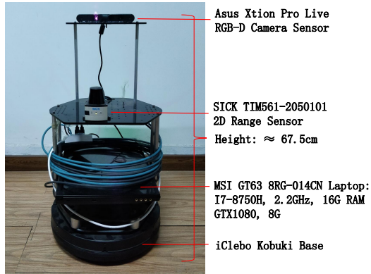
Fig. 4. The robot platform. TurtleBot 2 platform equipped with a RGB-D camera, a 2D range sensor and a Kobuki mobile base.
