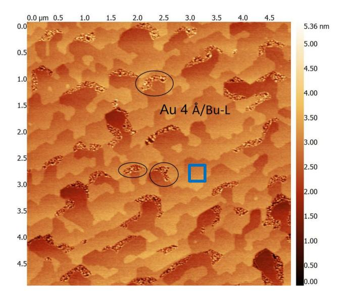
Figure S1. Atomic force microscopy (AFM) of substrates after Au deposition. (a) AFM topography of the Bu-L after 4 Å Au deposition (i.e. before Au intercalation at high temperature). The surface is smooth after deposition of Au (RMS roughness ~1 Å) in areas such as the one indicated by the blue rectangle. Au agglomeration only take place on the substrate areas where monolayer patches are present (circled areas). The height of SiC substrate steps is ~5 Å.
