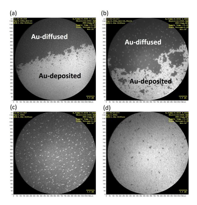
Figure S3. Low energy electron microscopy (LEEM) of Au-intercalated quasi-free-standing monolayer graphene on SiC ( $t_{Au} = 8$  Å). (a) LEEM image taken at the boundary of the deposited Au-deposited and Au-diffused areas. (b) The zoom in of (a) shows homogeneous morphology of quasi-free-standing monolayer graphene and bilayer graphene patches in the Au-diffused (c) and Au-deposited (d) areas.
