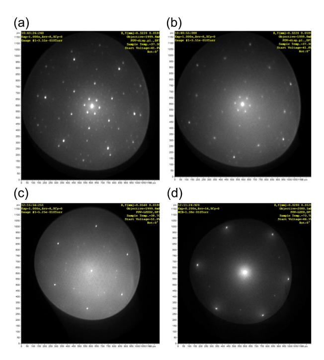
**Figure S4**. Low energy electron diffraction (LEED). (a) diffractogram of pristine Bu-L and (b) the Au-deposited area ( $t_{Au} = 8$  Å) before Au intercalation show the  $6\sqrt{3} \times 6\sqrt{3}$  R30 grid, which is the characteristic of Bu-L. After thermal intercalation, the  $6\sqrt{3} \times 6\sqrt{3}$  R30° grid disappear
