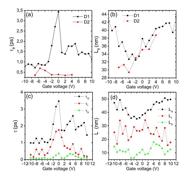
Figure S7. Weak localization analysis for Au intercalated quasi-free-standing monolayer graphene. (a) Phase coherence time in D1 and D2 obtained from the curvature of magneto conductivity at B = 0 and (b) corresponding phase relaxation lengths ( $L_{\phi}$ ) of D1 and D2. Scattering times  $\tau_{\phi}$ ,  $\tau_i$ , and  $\tau_*$  (c) and scattering lengths  $L_{\phi}$ ,  $L_i$ , and  $L_s$  of D1 (d) extracted from the best fits to the WL equation of monolayer graphene,<sup>1</sup>
