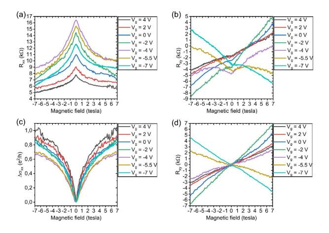
Figure S6 Magnetotransport in Au intercalated quasi-free-standing monolayer graphene.
