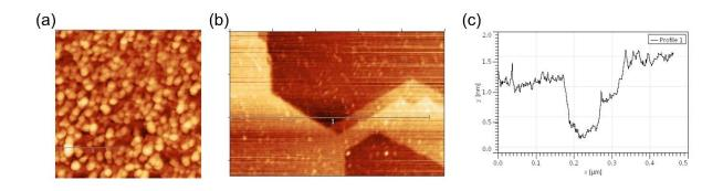
Figure S2. Atomic force microscopy (AFM) of Au-intercalated quasi-free-standing monolayer graphene on SiC ( $t_{Au} = 8$  Å). Atomic force microscopy image of the (a) Au-deposited area, and (b) the Au-diffused areas after thermal annealing at 850 °C. (c) Height profile in (b) showing atomically flat surface of intercalated surface.
