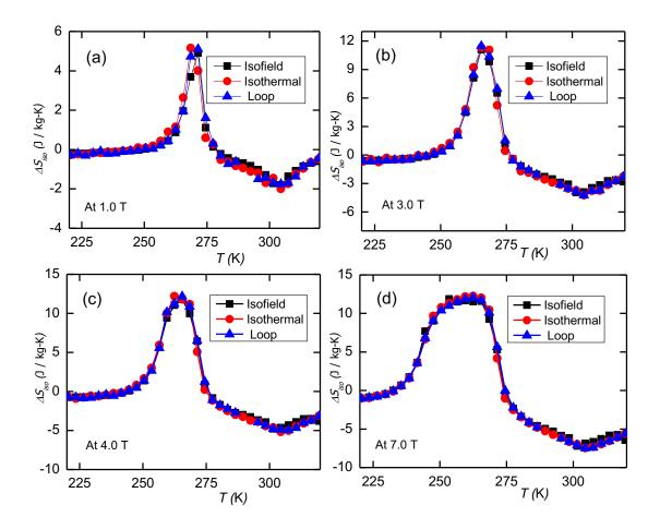
Figure 5. Comparison of isothermal entropy change  $\Delta S_{iso}$  as a function of temperature for the isofield, isothermal, and loop measurement protocols for Ni<sub>1.9</sub>Pt<sub>0.1</sub>Mn<sub>1.4</sub>In<sub>0.6</sub> at different applied field values (a) 1 T (b) 3 T (c) 4 T and (d) 7 T.
