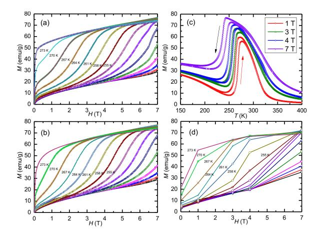
Figure 4. Magnetization measurement results for the  $Ni_{1.9}Pt_{0.1}Mn_{1.4}In_{0.6}$  (a) magnetic isotherms obtained from isothermal measurent protocol. (b) magnetic isotherms obtained from the loop measurent protocol. (c) isofield (M(*T*)) curves of  $Ni_{1.9}Pt_{0.1}Mn_{1.4}In_{0.6}$  at different field values. (d) magnetic isotherms extracted from isofield curves shown in (c).
