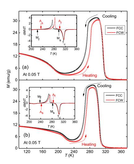
Figure 1. Temperature dependent magnetization curve of (a)  $Ni_2Mn_{1.4}In_{0.6}$  and (b)  $Ni_{1.9}Pt_{0.1}Mn_{1.4}In_{0.6}$  at H= 0.05 T. Insets show differential (d*M*/d*T*) curves for better presentation of transition and hysteresis.
