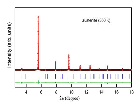
Figure 2. Le Bail refinement of SXRPD data of Ni<sub>1.9</sub>Pt<sub>0.1</sub>Mn<sub>1.4</sub>In<sub>0.6</sub> in austenite phase (350 K). The experimental peak profile, calculated peak profile and the difference are shown by black circle, red and green solid lines, respectively. The blue lines represent the Bragg's peak positions.
