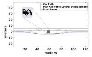
Fig. 2: The vehicle must go around the obstacle to the left or to the right. This is represented by two new lanes to follow. The vehicle in this situation chooses to follow the right lane.
