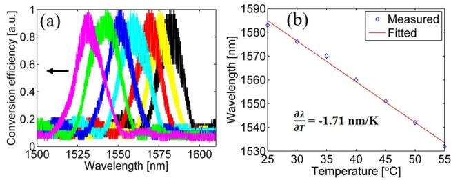
**Fig. 5.** (a) Measured phase matching curves of the LNOI waveguide blue shifted as the temperature increases from 25°C to 55°C at 5 °C step. (b) Temperature dependency of the QPM wavelength, with the tunability fitted to be -1.71 nm/K.
