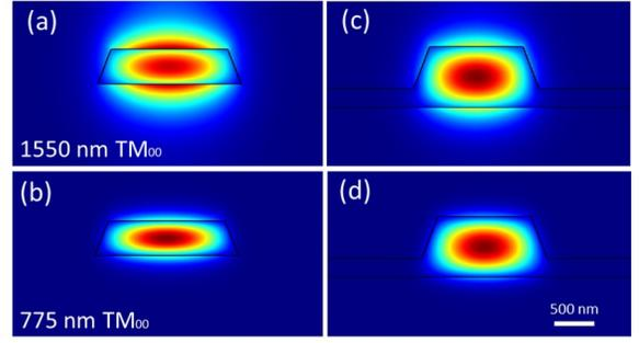
**Fig. 1.** Simulated profiles for the 1550-nm and 775-nm quasi-TM<sub>00</sub> modes. The waveguide cross section  $400 \times 1850$ nm (height and top) for (a) and (b), and  $700 \times 1500$ nm for (c) and (d). For latter one, the etched depth is 480 nm, so that a layer of 220 nm LN slab is remained. The simulated sidewall angle in is  $62^\circ$  for all figures.
