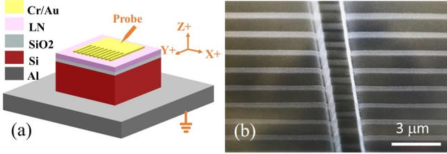
**Fig. 3.** (a) Schematic of periodic poling on the Z-cut LNOI wafer placed on an aluminum hot plate. (b) SEM image of a PPLN waveguide with 3.8  $\mu\text{m}$  poling period. The fringe pattern is formed after hydrofluoric (HF) acid etching and indicates good uniformity along the propagation direction.
