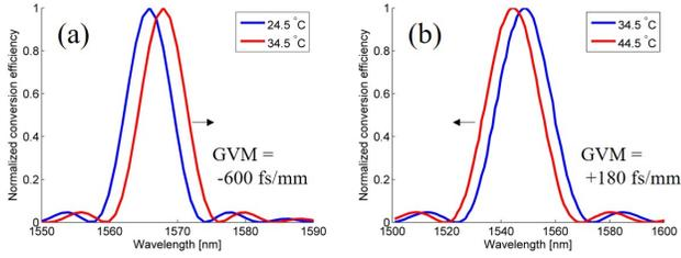
**Fig. 2.** Simulated phase matching curves of Waveguide 1 (a) and Waveguide 2 (b) under different temperatures. Waveguide 1 has a negative GVM (-600 fs/mm) and red shifts at 0.2 nm/K. Waveguide 2 has a positive GVM (180 fs/mm) and blue shifts at 0.6 nm/K.
