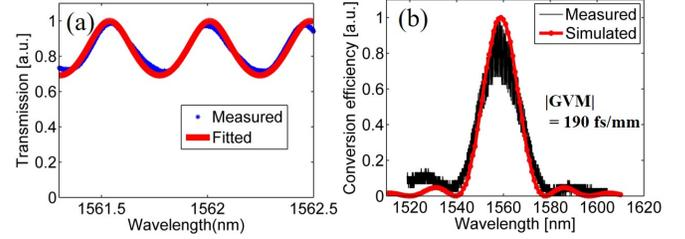
**Fig. 4.** (a) The spectra of Fabry-Perot resonances formed by the LNOI waveguide and its two polished facets. (b) Measured phase matching curve at  $T = 45^\circ\text{C}$ . The extracted GVM magnitude is 190 fs/mm. The device length is 1-mm long.
