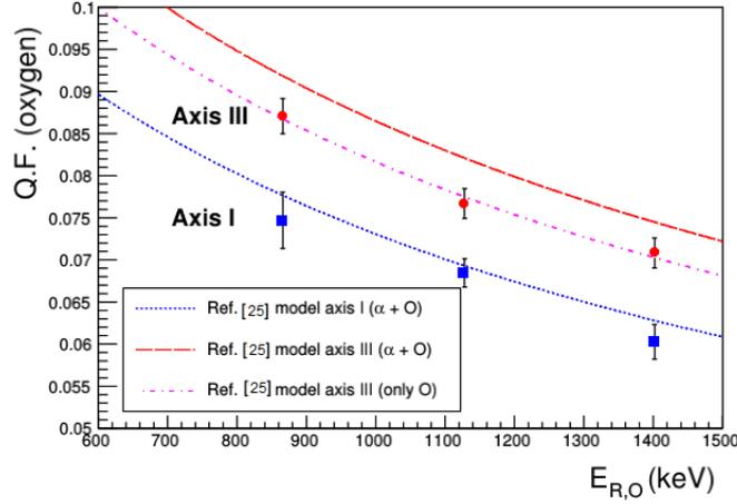
**Figure 7.** Quenching factors for oxygen nuclear recoils in  $\text{ZnWO}_4$  for the crystal axes I and III as function of the expected recoil energies  $E_{R,O}$ . In the plot the expected behavior of quenching factor for the two crystal axes of the model of Ref. [25] are also reported; they have been obtained by fitting the data of the  $\alpha$ 's and oxygen recoil data together, and oxygen recoil data only.
