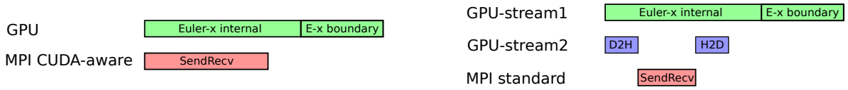
Figure 8: Sketch of asynchronous time-lines for the evaluation of convective fluxes: internal fluxes evaluation ( Euler-x internal ), boundary fluxes evaluation ( E-x boundary ), host-to-device transfers ( H2D ), device-to-host transfers ( D2H ), MPI communications ( SendRecv ). CUDA-Aware MPI based time-line is shown on the left while standard MPI time-line is provided on the right.
